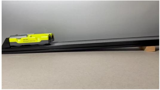
The sensor cart's plunger launches the cart. It then coasts up and down the incline.
