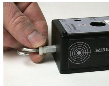
*The hook connected to the force sensor*
