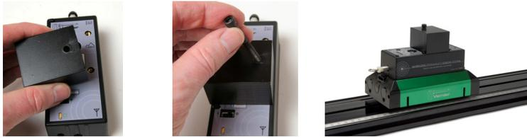
**Important:** Do not use any screw that would intrude more than 8 mm into the threaded hole. This could damage the internal electronics of the WDSS.
