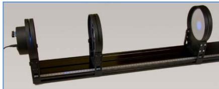
The three-color LED illuminator contains a high output RGB LED whose three single-color components are separately regulated by three potentiometers mounted on the back of the housing.
