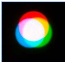
For subtractive color mixing, a diverging cone of light is produced and the screen adjusted until it is evenly illuminated with white. Typical positions have the lens 5 cm from the light source and the screen 30 cm from the lens.
