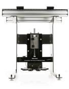
The Structures & Materials Tester is equipped with a force sensor (rated to 1000~N) and an encoder to measure displacement (1  $\mu$ m resolution). Using both sensors, you can record maximum loads, as well as load versus displacement characteristics, so students can evaluate deflection, stress, and strain.
